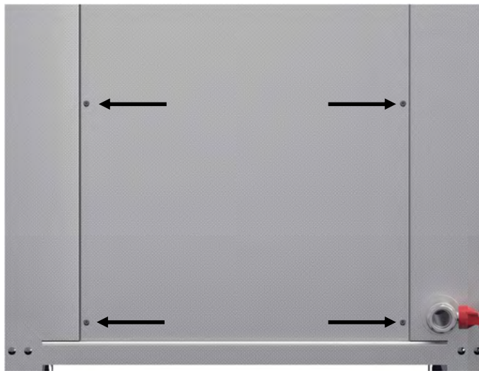
Fig. 9.5.1. Position of the 4 Allen screws
