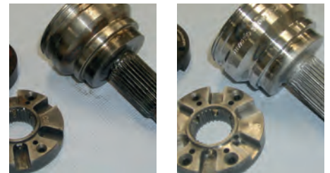
Removal of oxidation and other contaminants
