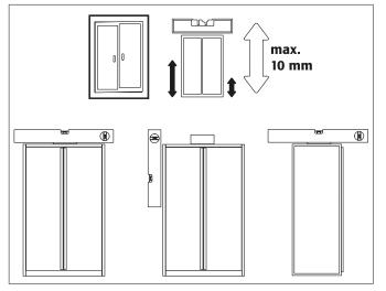
If necessary, level the cabinet by adjusting the support feet.
