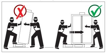
When the cabinet touches the ground, support it so that the pallet can be removed.
