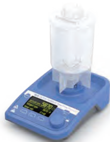
ULTRA-TURRAX® Tube Drive Power control Ident-No.: 0025005981
