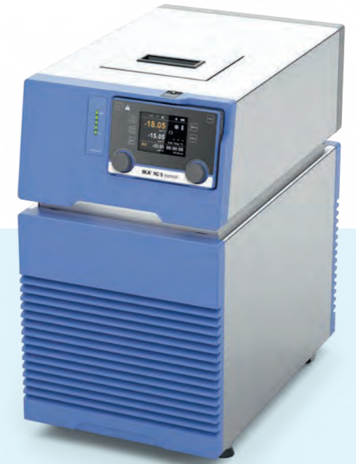
RC 5 control Recirculating chiller
