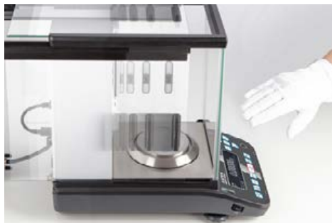
Automatic sliding doors, which can be opened and closed using sensors
