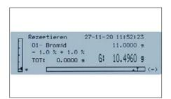
Convenient recipe-weighing: with the recipe database, in which up to 99 recipes can be stored, each with up to 20 recipe ingredients with name and target value
