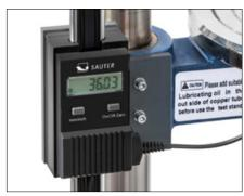
Distance measurement directly in machines or sites with RS-232 interface
