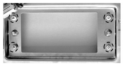
7. Place the relay output with the holes on the screw pins
