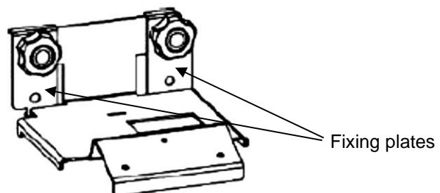
10. Hook the fastening plates onto the cable compartment and tighten them with the knobs [9] a little more than hand-tight.
