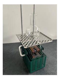
• The rods can accommodate laboratory clamps for holding test tubes.
