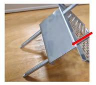
Screw the rods into the nuts on the back of the MICROBIO:
