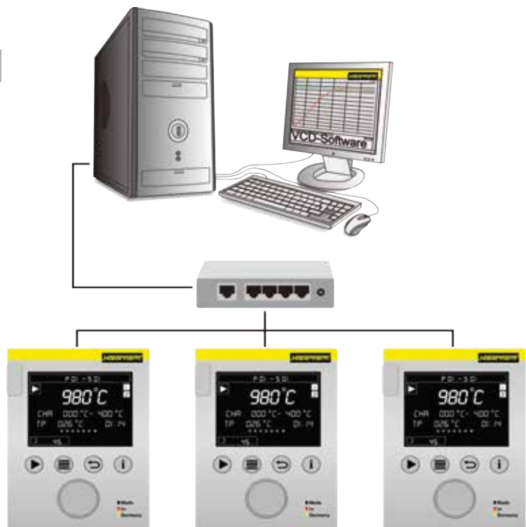
Example lay-out with 3 furnaces
