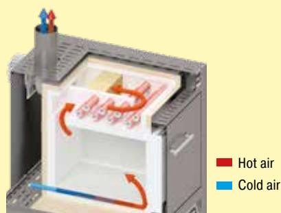
Schematic presentation of air circulation in ashing furnace L 24/11 BO
