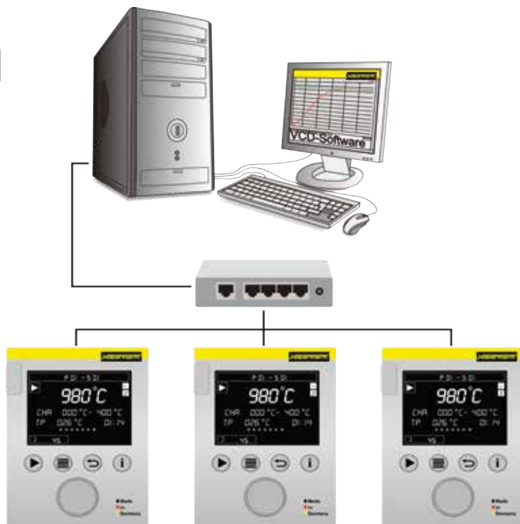
Example lay-out with 3 furnaces
