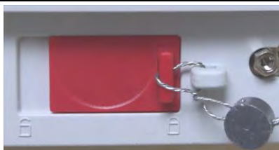
Locked with Wire Seal
