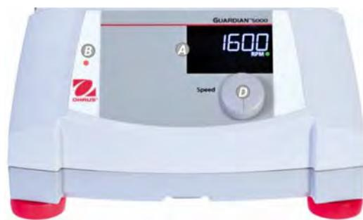
**A. Display Screen****B. Standby Indicator****D. Knob:** Controls speed**F. Fuse**
