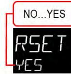
7. Press and hold the left knob (C) until the unit beeps to confirm the Reset setting.
