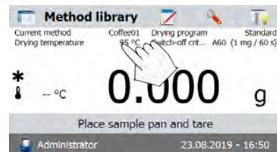
MB120 moisture analyzer features SmartGuide™ function. It can automatically generate suitable test method for your samples.
