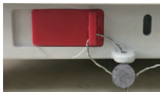
Locked with Wire Seal
