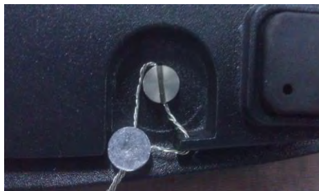
Locked with Wire Seal
