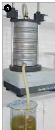
4 Processus de tamissage humide (rinçage + vibration)
