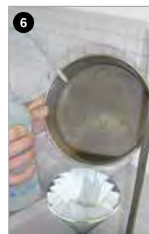
4 Processus de tamissage humide (rinçage + vibration)
