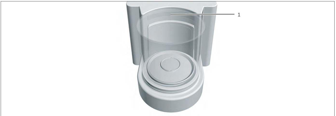
Fig. 7: Weighing compartment lighting (example)
