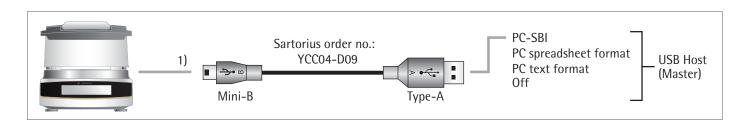
(1) USB Connection as PC Keyboard without Additional Driver via a PC with Table or Spreadsheet Editor (e.g., Microsoft<sup>®</sup> Office or OpenOffice)
