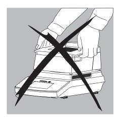
Never lift and carry the analyzer by its heating module.
