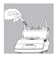
Clean the heating element and temperature sensor with a weak solvent such as ethanol.
