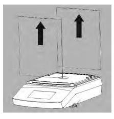
8) Pull out the front and rear glass panels (upwards).
