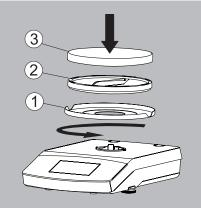
3) Install the pan support (1) and weighing pan (2).
