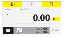
The Checkweighing application appears. The set thresholds are displayed under Min and Max.
