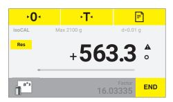
▷ The weight of the sample is multiplied by the entered factor, and the result is displayed.
