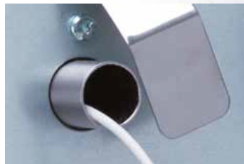
Dedicated access port (18 mm diameter) allows the introduction of independent sensors
